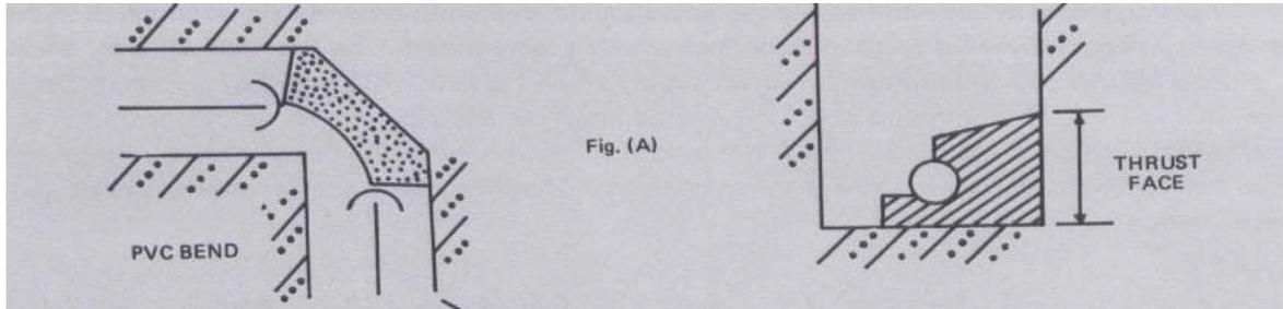
The design of uPVC pipes provides a safety factor of 2.1 after a life of 50 years at maximum working pressure. In designing thrust blocks it is logical to apply a similar factor of safety after calculating thrust forces on the maximum foreseeable line pressure.
